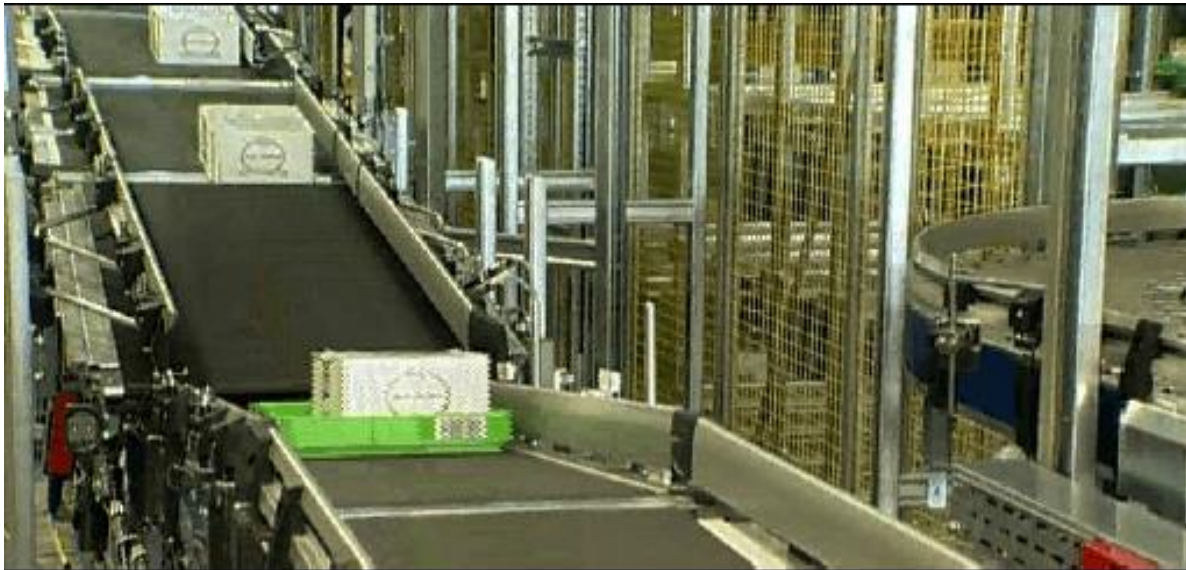
Photograph of individual cases placed into trays for intermediate storage prior to cage build
