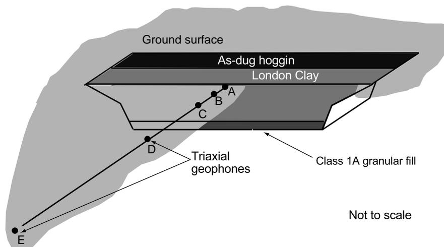
**Figure A6 Schematic arrangement of test structure**
