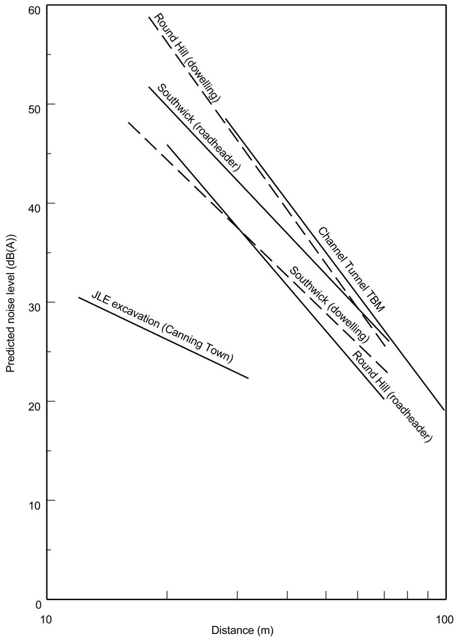
**Figure 48b** Upper-bound lines fitted to calculated groundborne noise levels for tunnelling operations
