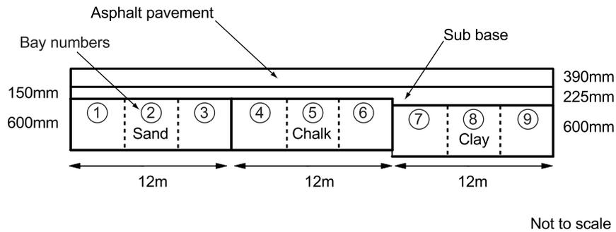
Figure 21 Section through trial road
