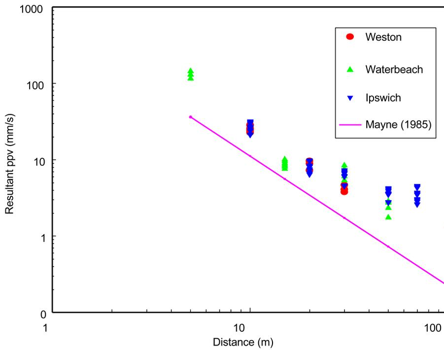
**Figure 44** Vibration data from the high speed dynamic compactor reported by Allen (1996) compared with ppv predicted for the 7t tamper dropped from 1.2m using Mayne's equation (1985)
