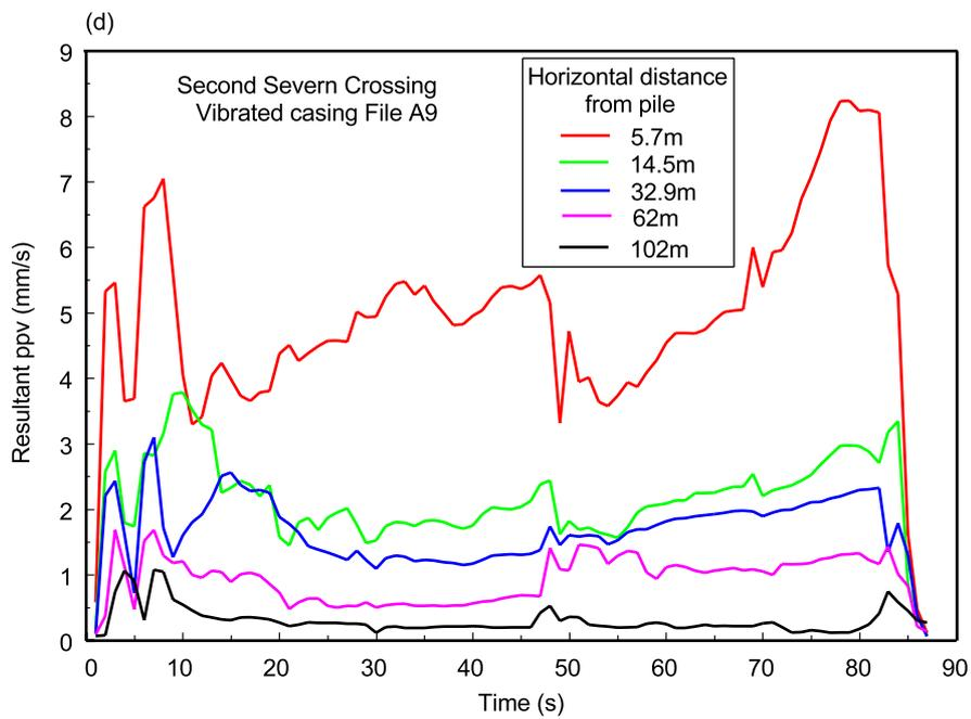
**Figure 40 (continued)** ppvs measured during vibratory casing driving at (c) the Dee Crossing and (d) the Second Severn Crossing
