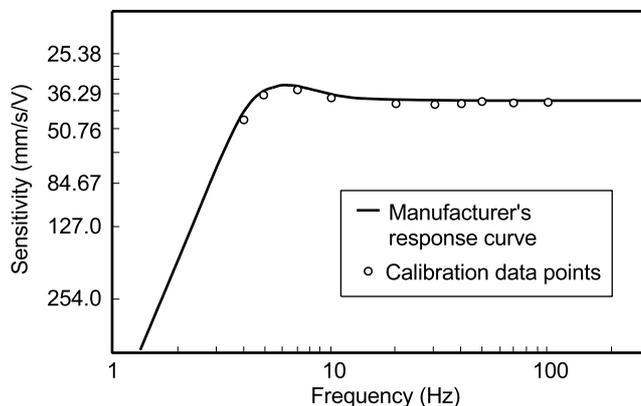
Figure 7 Measured geophone response curve
