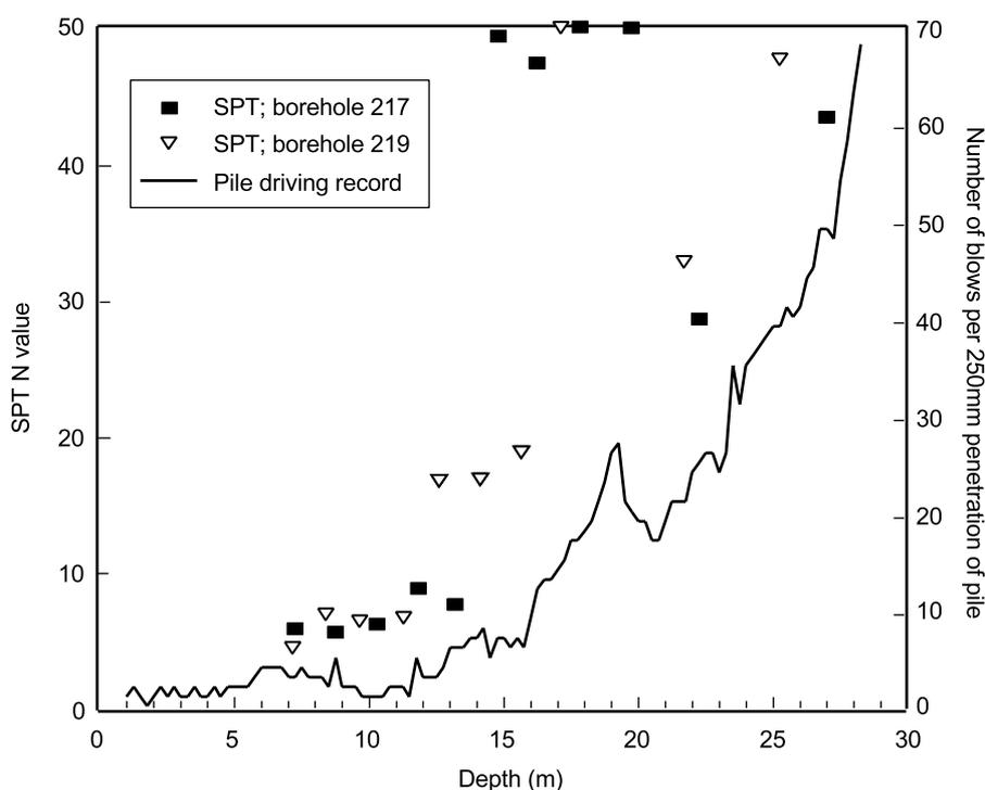
Figure 31 SPT and pile driving data from the A47 piling site
