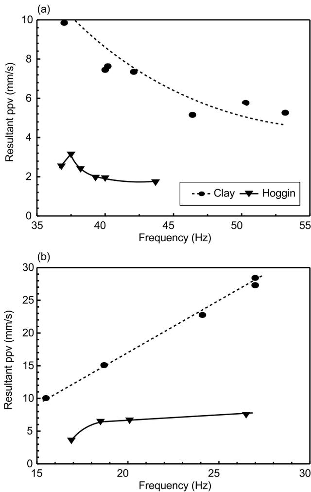
**Figure 14** Effect of frequency on ppv for two vibrating rollers: (a) the Ingersoll-Rand DD65 (b) the Ingersoll-Rand DS150
