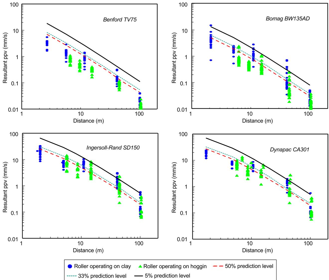
**Figure 28** Equation 10 fitted to data from the controlled trial
