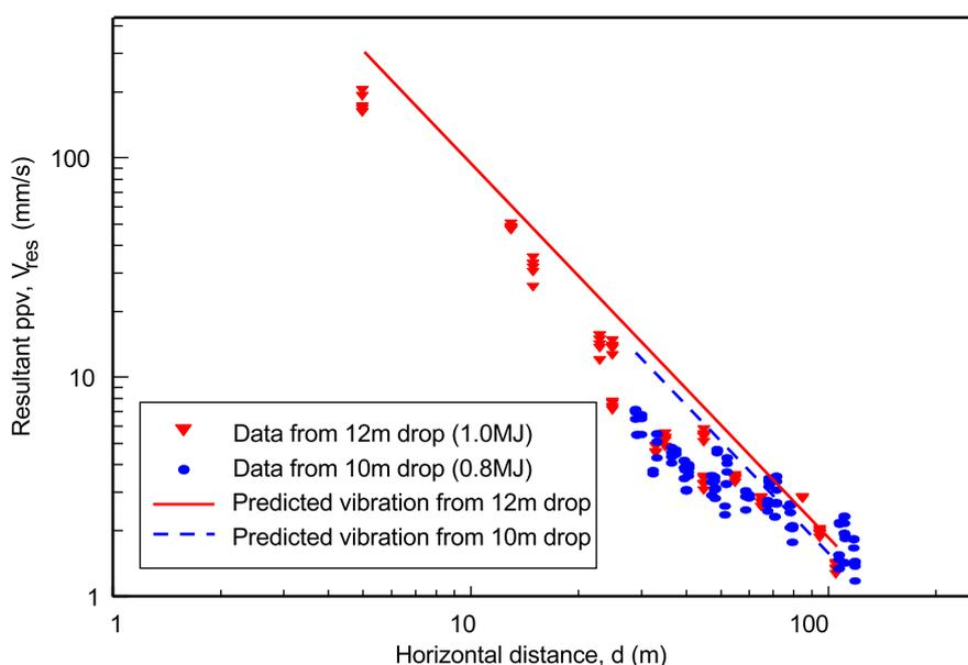
**Figure 43** Data from dynamic compaction using an 8.5t tamper at the Coventry site compared with vibration predicted using Mayne's equation (1985)
