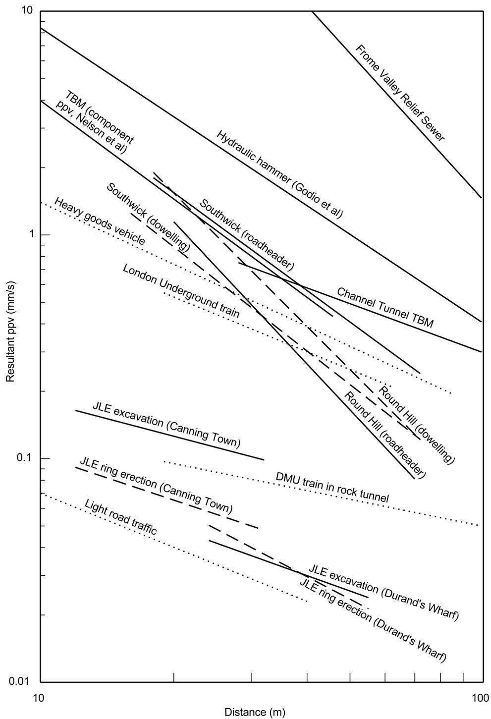
**Figure 46b** Upper-bound lines for blasting data from the Frome Valley sewer compared with those for various operations
