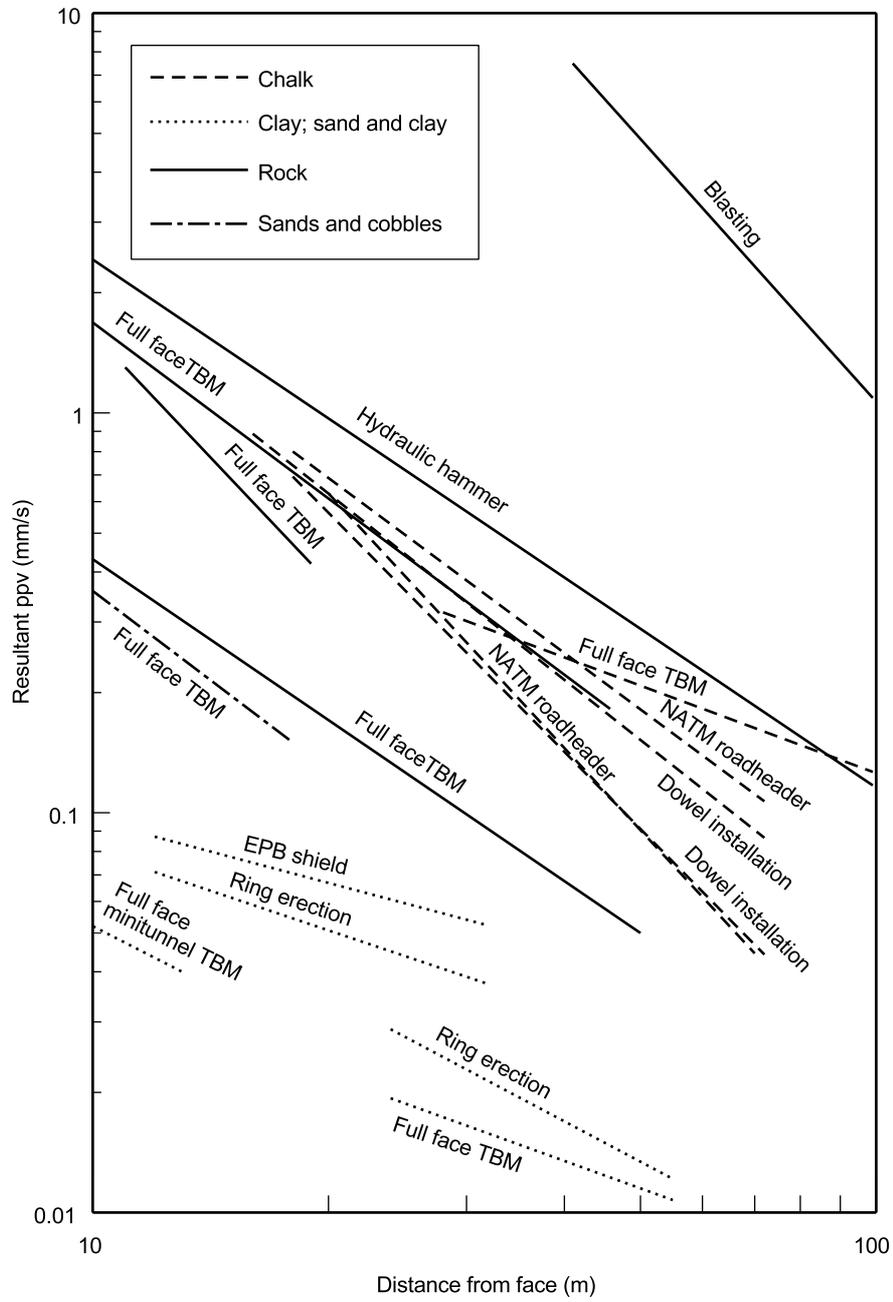
**Figure 49** Ground vibration data from tunnelling operations classified according to geology
