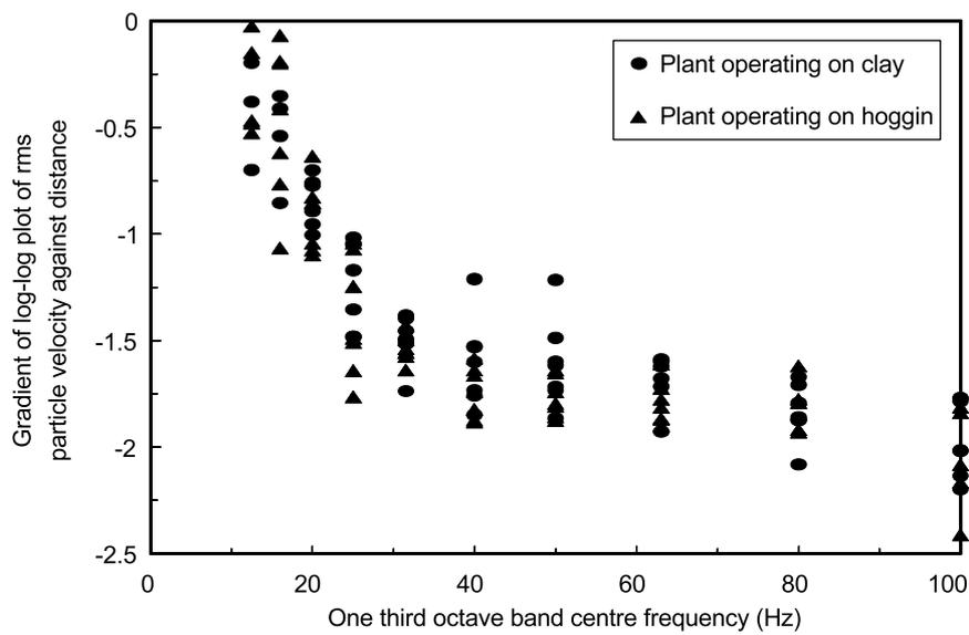
**Figure 25** Attenuation vs. frequency for PV data separated into third octave bands
