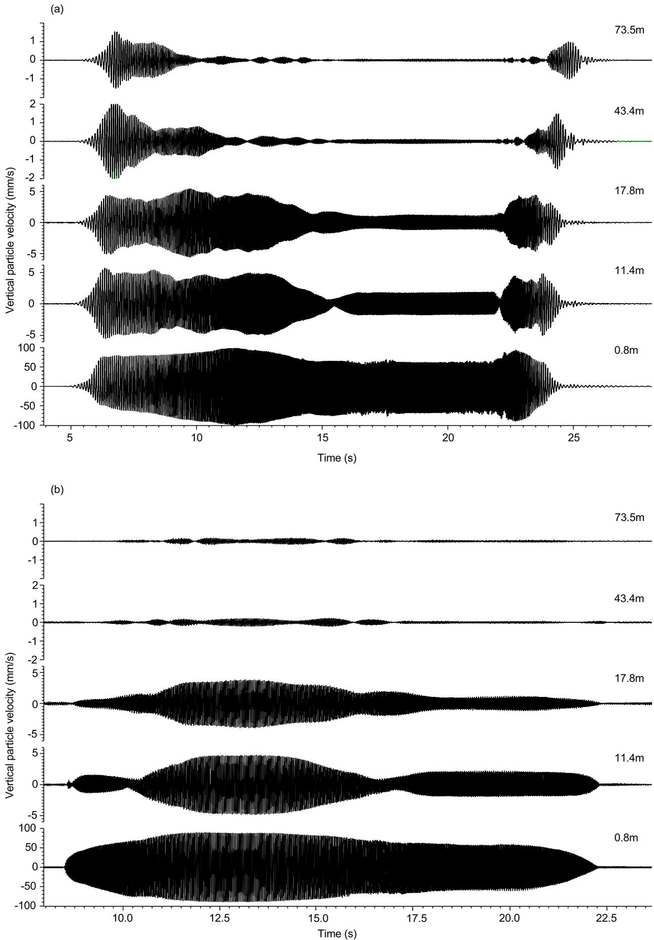
**Figure 41** Comparison of vibration arising at various distances from 14RF vibrodriver at Radstock operated (a) conventionally and (b) in resonance-free mode
