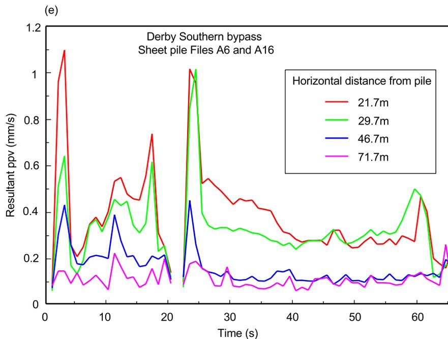
**Figure 40 (continued)** ppv from vibratory driving of sheet piles at the Derby Southern Bypass
