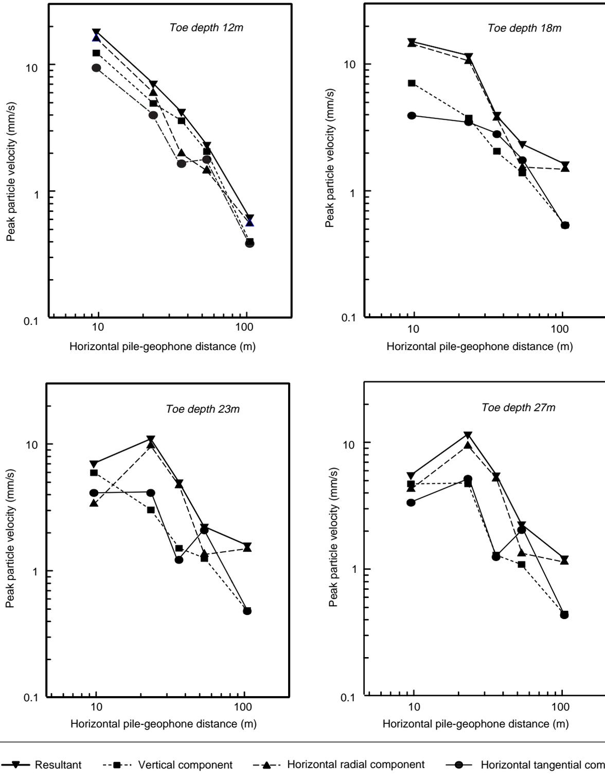
**Figure 34** Change in shape of the attenuation curve with pile toe depth ( $L$ ) when plotted against horizontal distance ( $d$ ) from the pile during the driving of a pile at the A47 site
