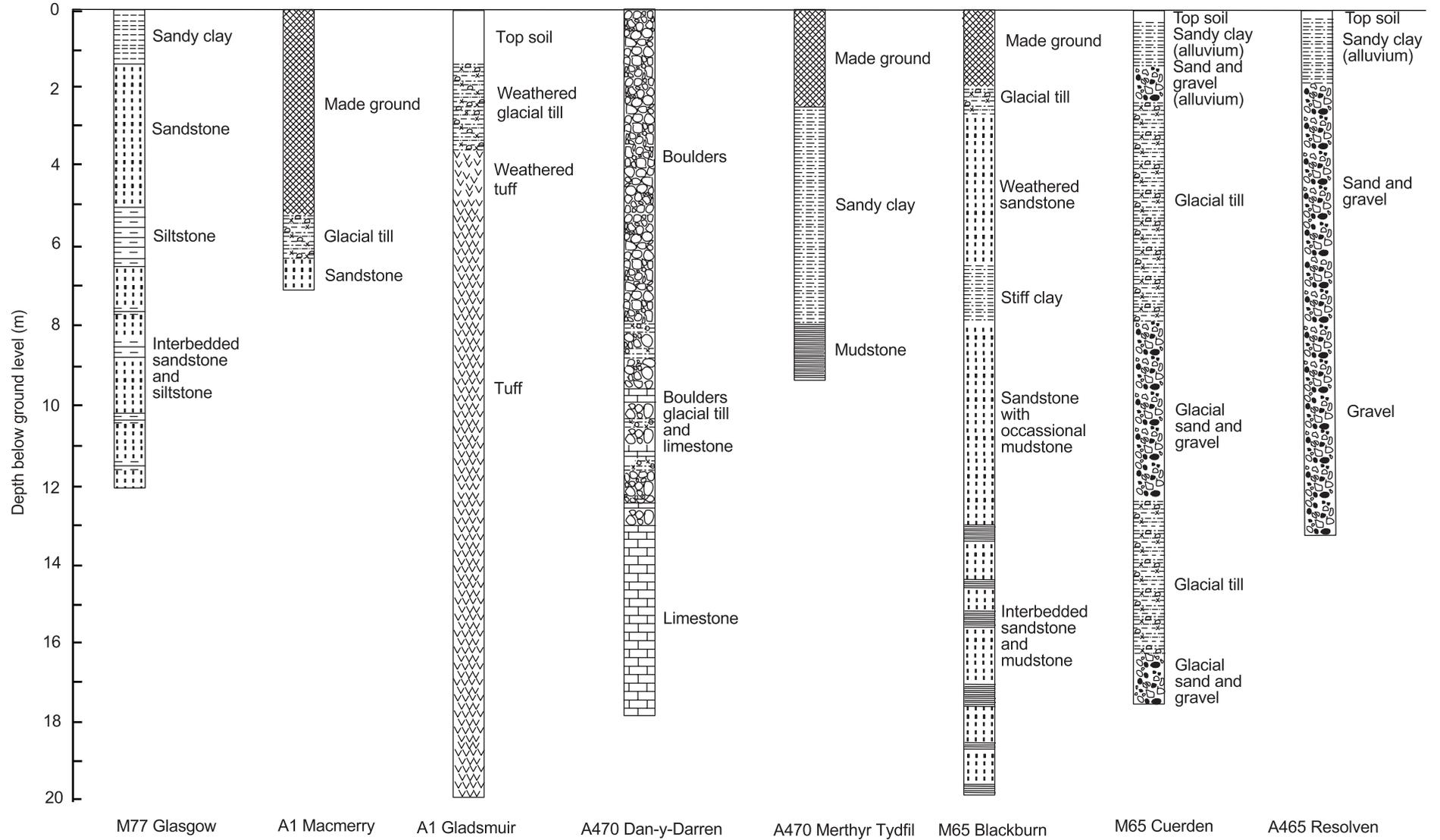
**Figure 9a** Simplified geological profiles for eight of the sixteen sites on which data from vibrating rollers were acquired
