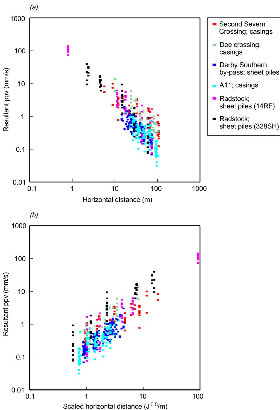
**Figure 37** Field data from all vibrodriving sites in the current study plotted against (a) the horizontal distance from the pile and (b) the horizontal distance scaled by the nominal energy per cycle of the vibrodrivers
