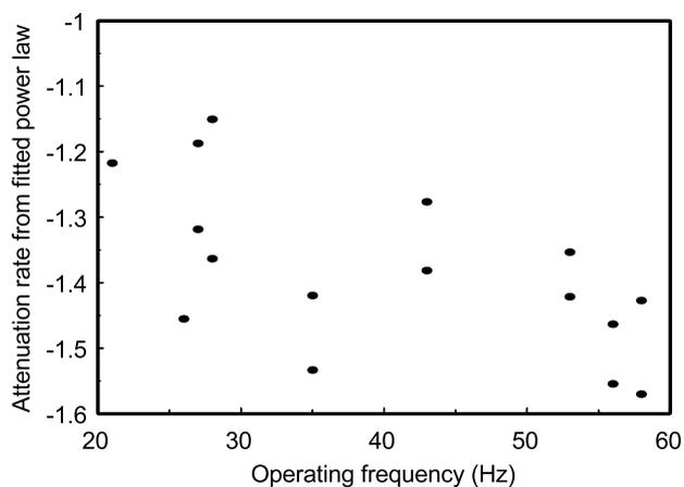
**Figure 23** The relation between the operating frequency and the rate of attenuation of vibration for compaction plant operated during the roller trial
