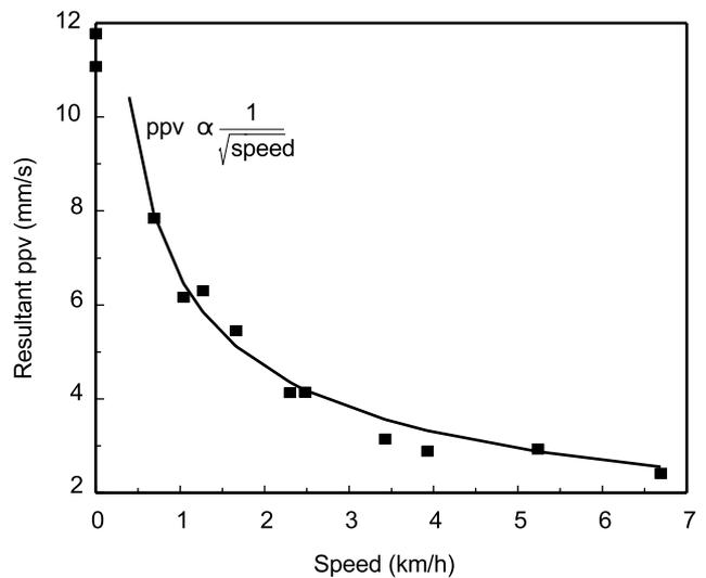
**Figure 17** Effect of travel speed on the ppv recorded at a distance of 2.1m during operation of the Bomag BW161AD roller
