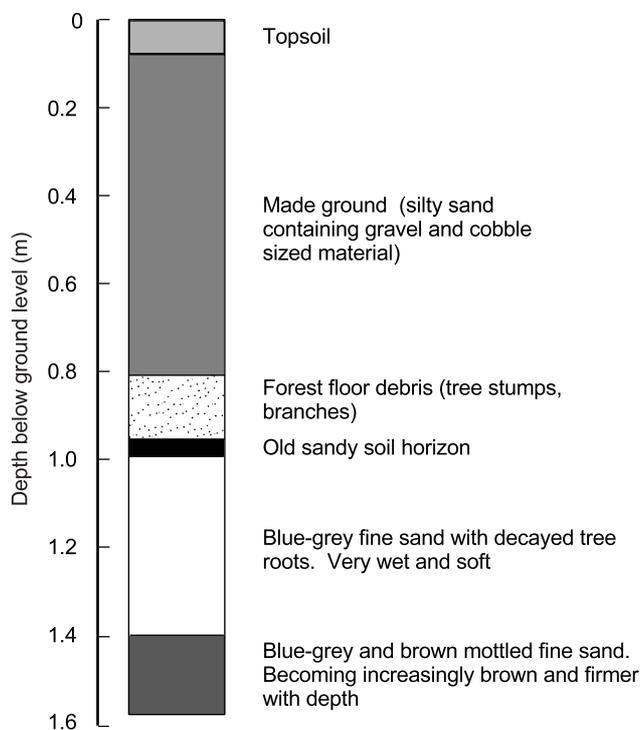
Figure A2 Soil profile at TRL trial site
