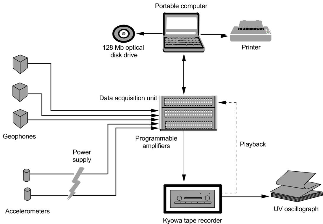
**Figure 6** Schematic of data acquisition equipment
