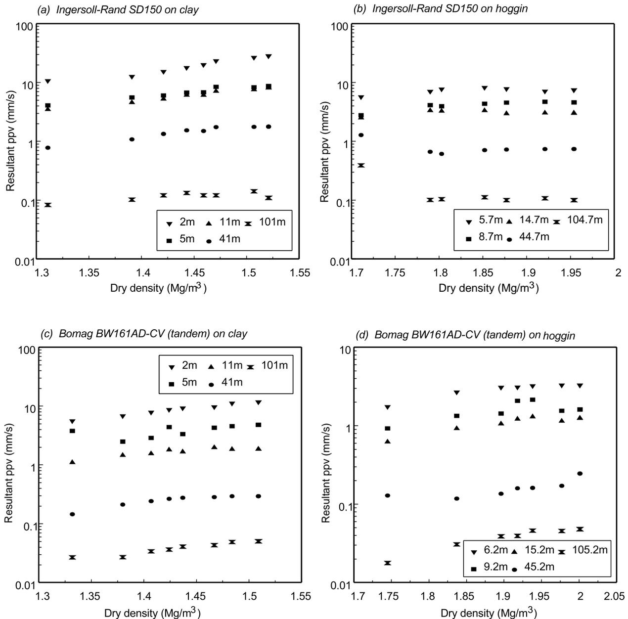
**Figure 20** The effect of dry density of each fill material on the peak particle velocity recorded at each geophone. (a) and (b) are data from a single drum vibrating roller, (c) and (d) are data taken from a tandem vibrating roller
