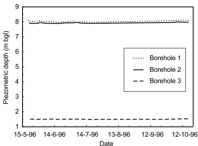
**Figure A5** Piezometer data for the duration of the TRL field trial
