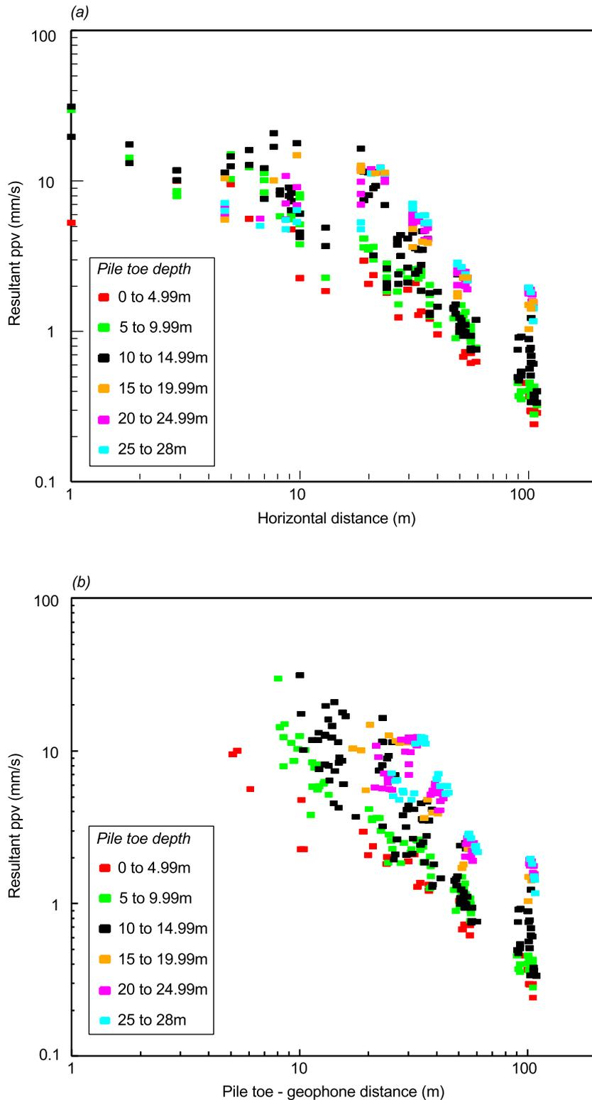
**Figure 30** Ground vibration data from the A47 piling site plotted against (a) horizontal distance from the pile and (b) slope distance from the pile toe
