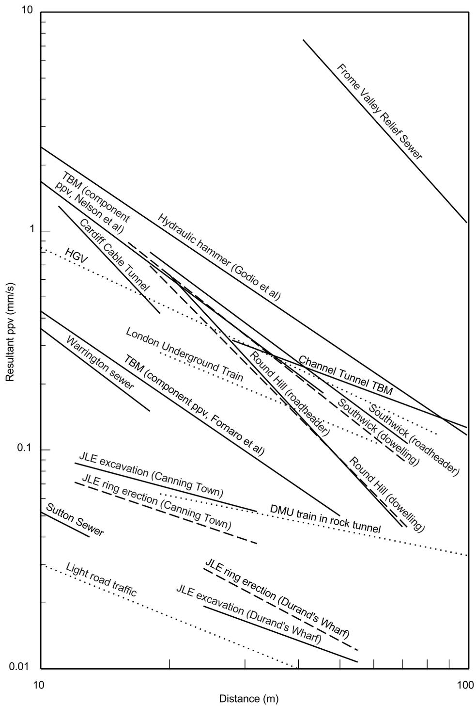
**Figure 46a** Regression lines for blasting data from the Frome Valley sewer compared with those for various tunnelling operations
