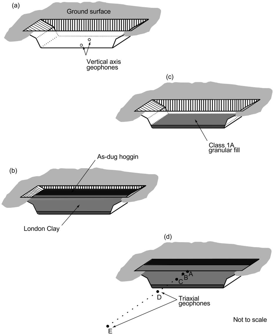
**Figure A3** Construction sequence of TRL trial earthwork
