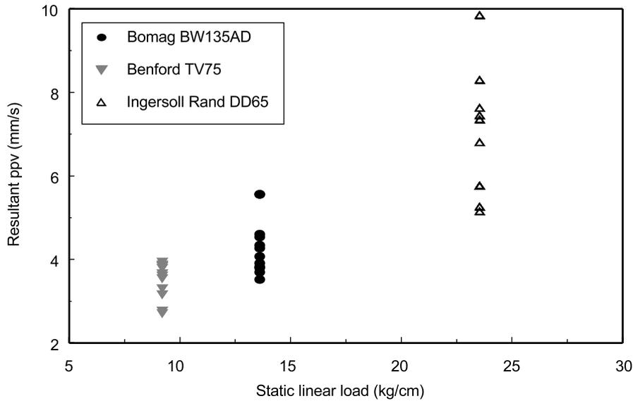
**Figure 16** Effect of static linear load on ppv for three tandem rollers
