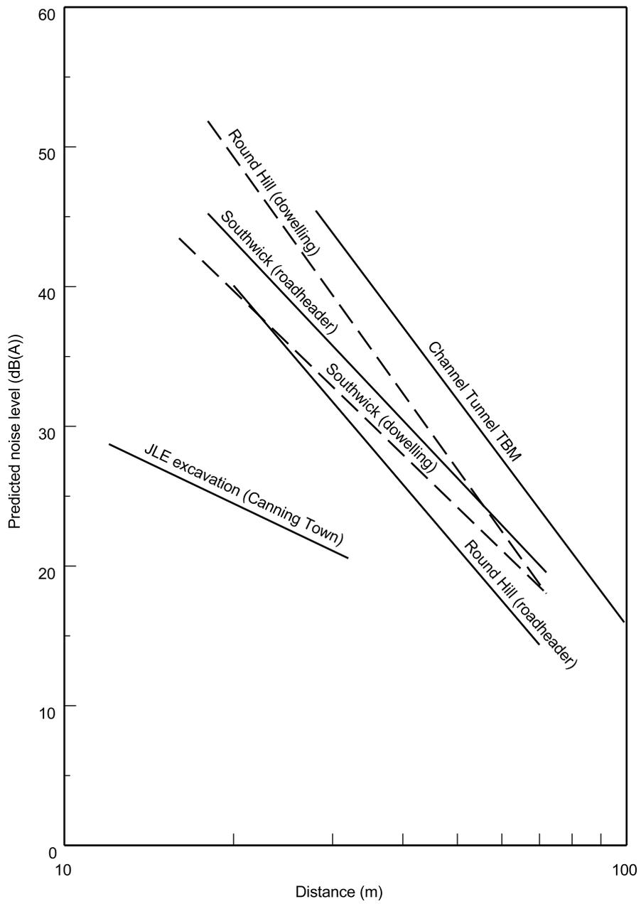
**Figure 48a** Regression lines fitted to calculated groundborne noise levels for tunnelling operations
