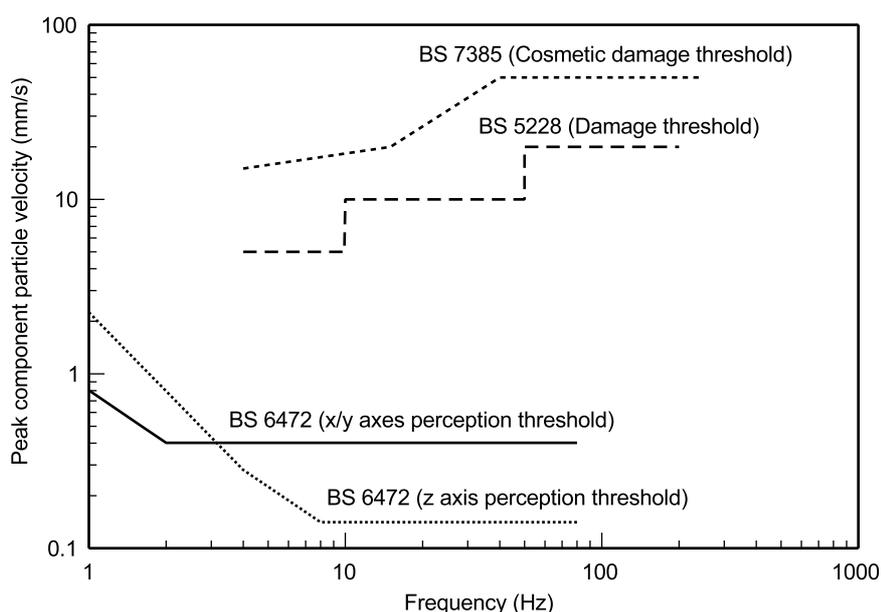
**Figure 3** Thresholds provided by British Standards for human perception and damage to domestic structures by transient vibrations
