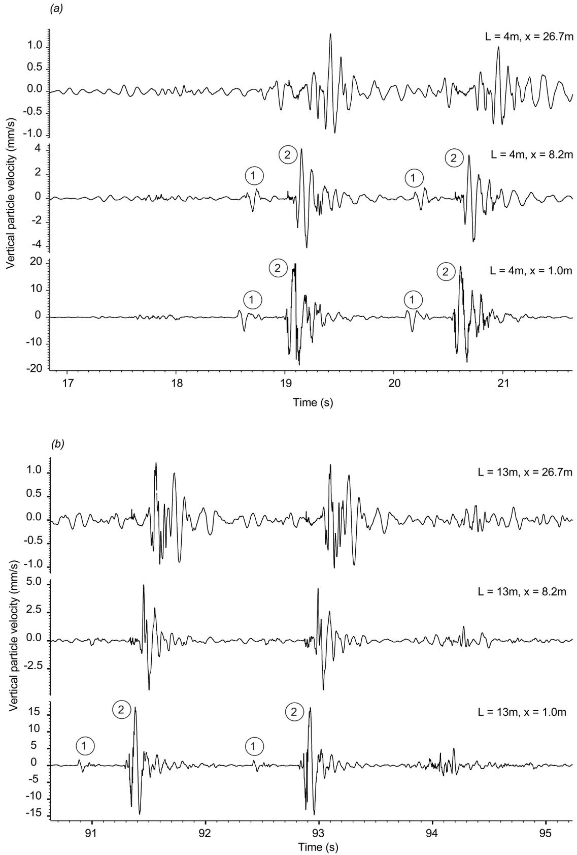
**Figure 33** Vertical component of vibration at the A47 site from (a) the first two impacts of driving the lower section of a pile using the maximum nominal energy (toe depth approximately 4m) and (b) the end of driving (toe depth approximately 13m). The traces show a relatively low amplitude event (1) arriving approximately 0.5s before the main event (2)
