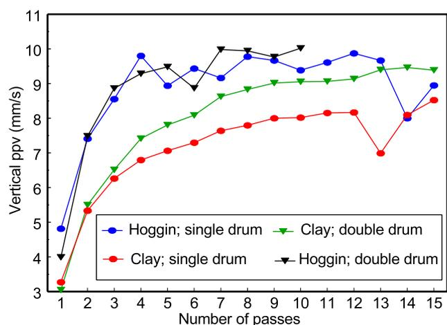
**Figure 13** Increase in ppv recorded by the vertical uniaxial geophones buried beneath the test structure with increasing number of passes of the Bomag BW161AD-CV Variomatic roller
