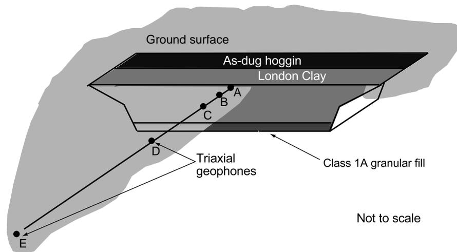
**Figure 12** Schematic arrangement of test structure
