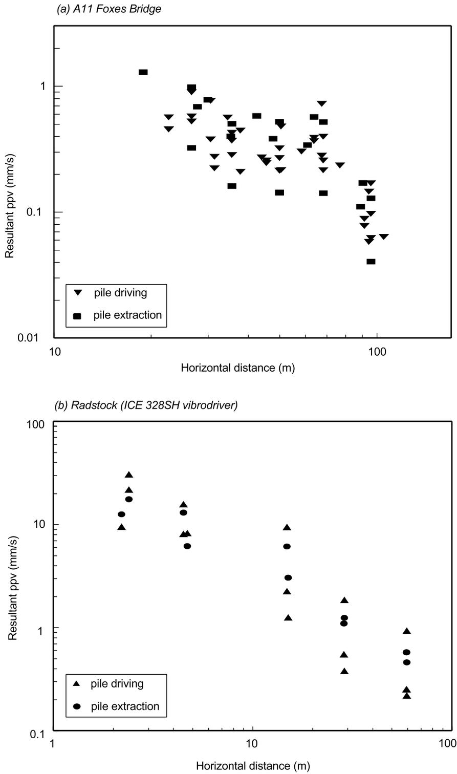
**Figure 39** Ground vibration data from the vibratory driving and extraction of piles at (a) the A11 Foxes Bridge site and (b) Radstock, using the ICE 328SH vibrodriver
