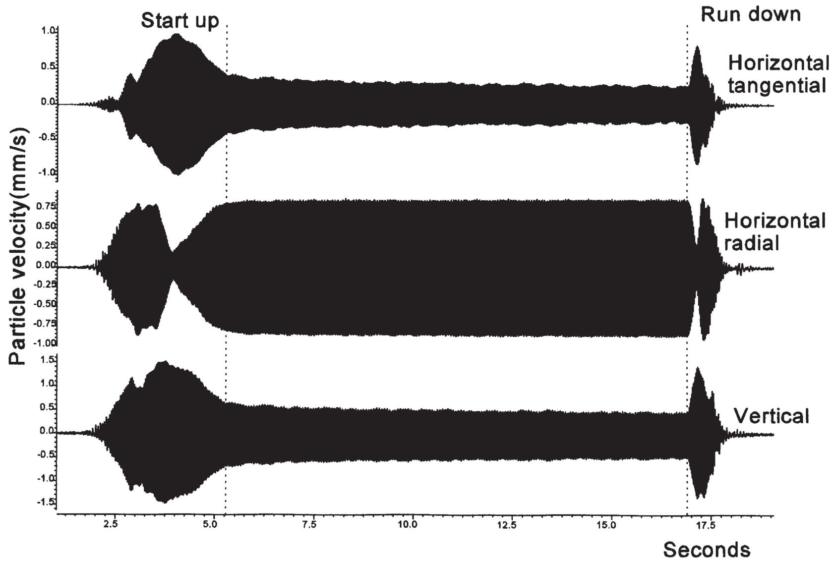
Figure 8 Signal from a vibrating roller, showing startup, steady state operation and stopping
