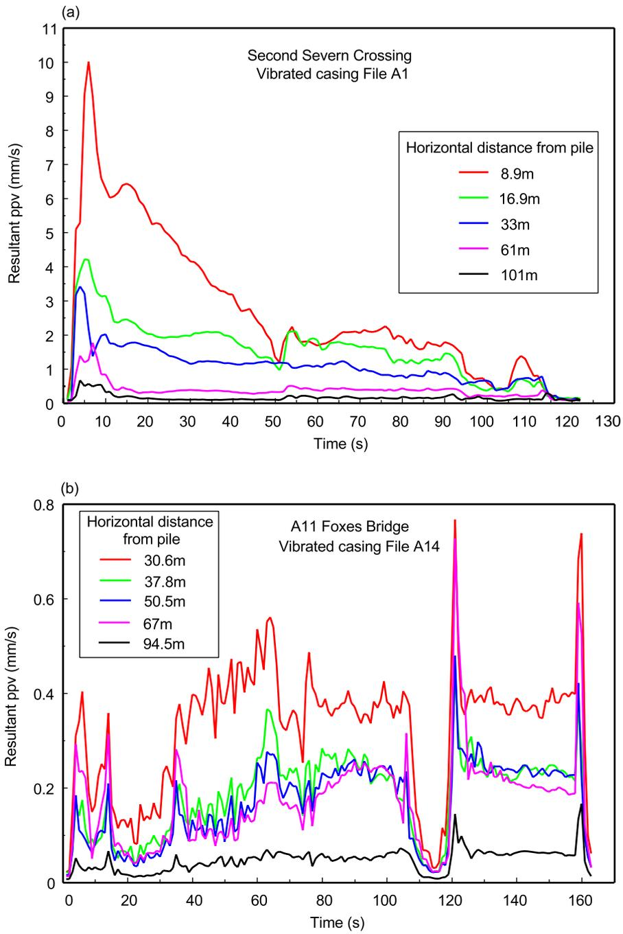
**Figure 40** Plots of ppv vs time during (a) pile extraction at the Second Severn Crossing and (b) driving at the A11 site
