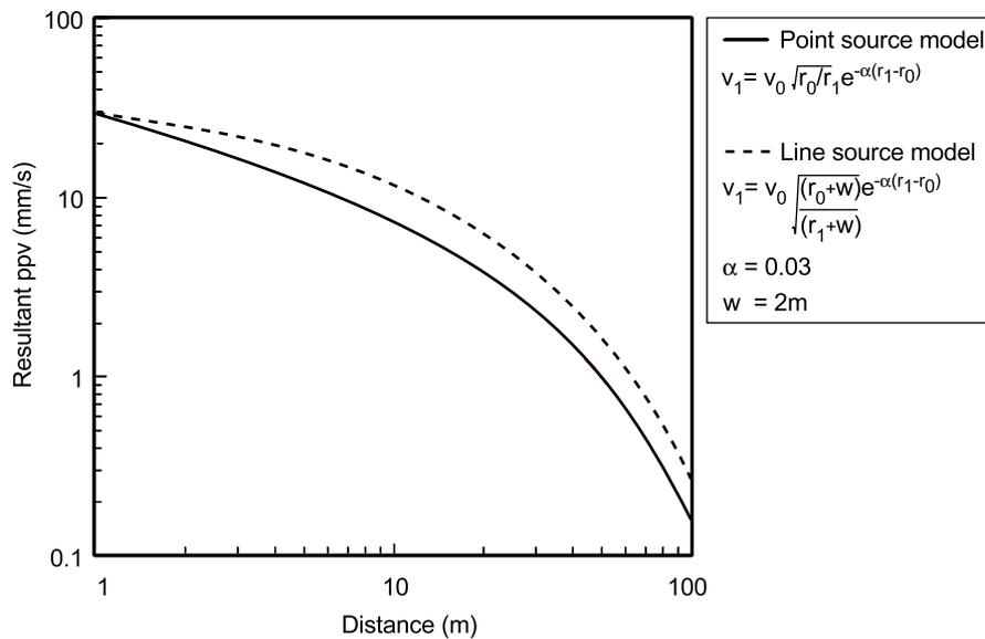
**Figure 27** Attenuation described by the relation proposed by Mintrop (1911) for a point source and the effect of assuming a 2m long linear source of vibration
