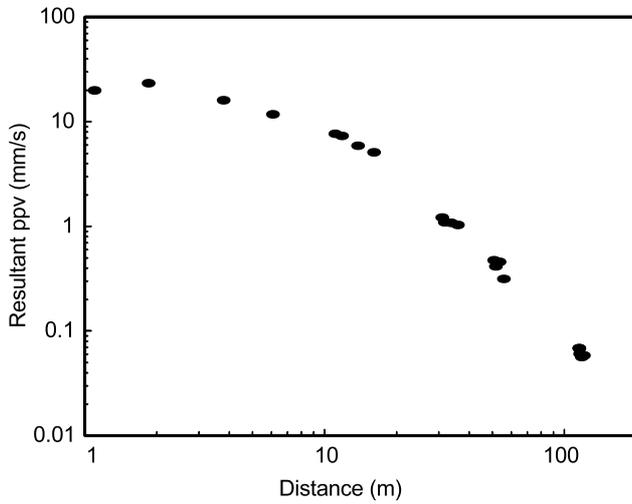
**Figure 26** Attenuation curve for vibration from a Bomag BW161AD operated on natural ground
