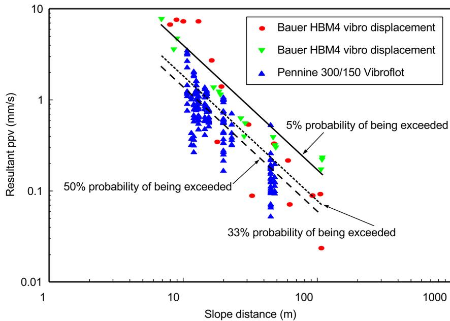
**Figure 45** Vibration caused by vibratory ground treatment and the proposed prediction limits
