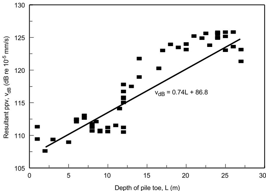
**Figure 32** Relation between vibration level at a distance of 100m or more from the pile and the pile toe depth at the A47 piling site
