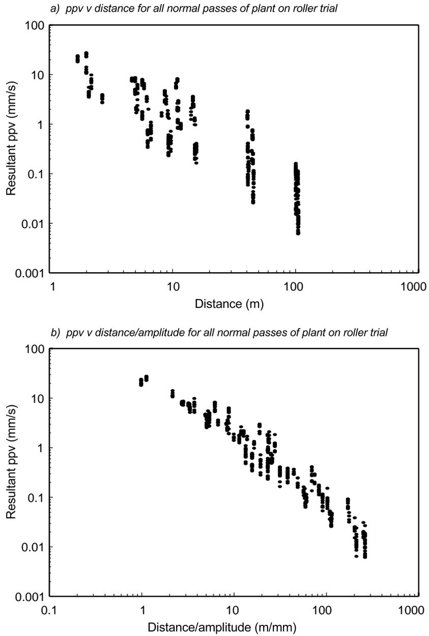
**Figure 11** The effect of normalising vibration data from the roller trial by the nominal drum amplitude
