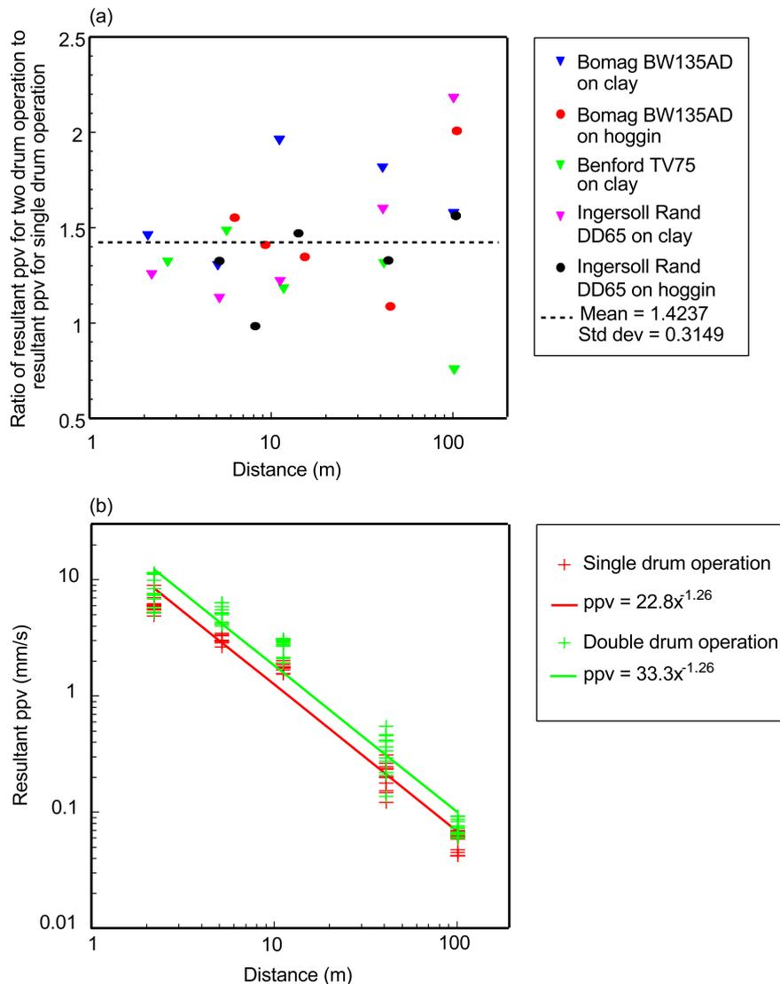
Figure 18 Effect of the number of vibrating drums on the level of groundborne vibration
