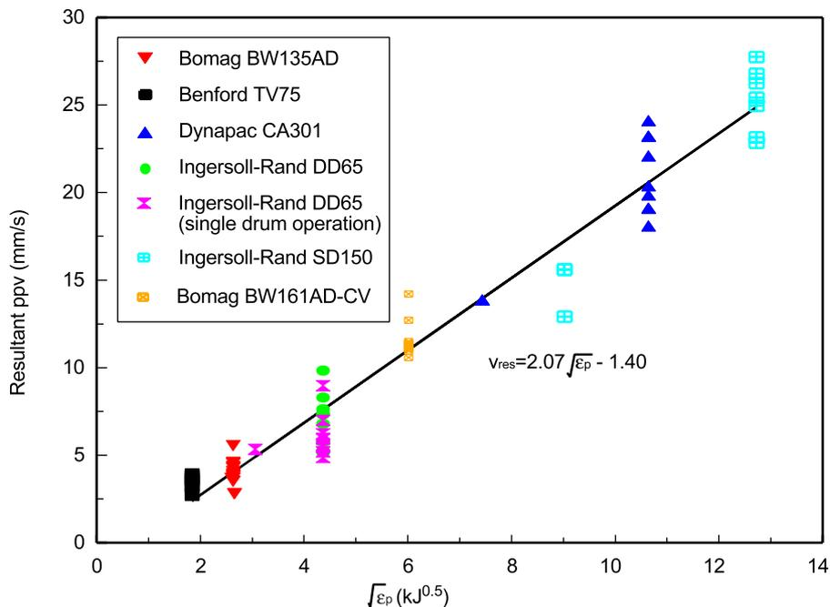
**Figure 19** Relation between the ppv recorded at Geophone A during the roller trial and a function of nominal amplitude, static linear load and drum width
