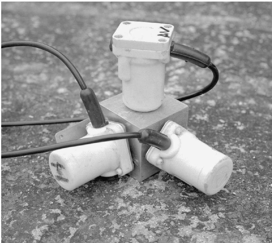
**Plate 3** Three geophones mounted orthogonally on a cube
