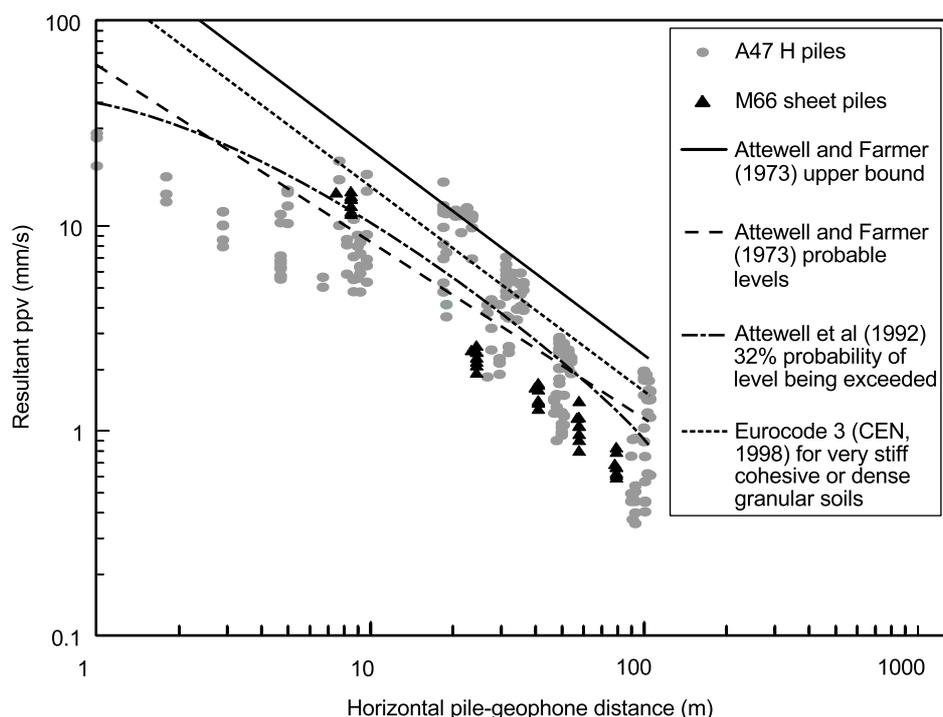
Figure 29 Current piling predictors plotted with TRL data from two sites
