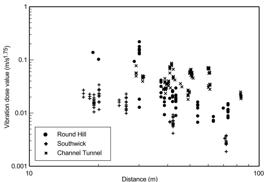
**Figure 47** Calculated vibration dose values for tunnelling operations
