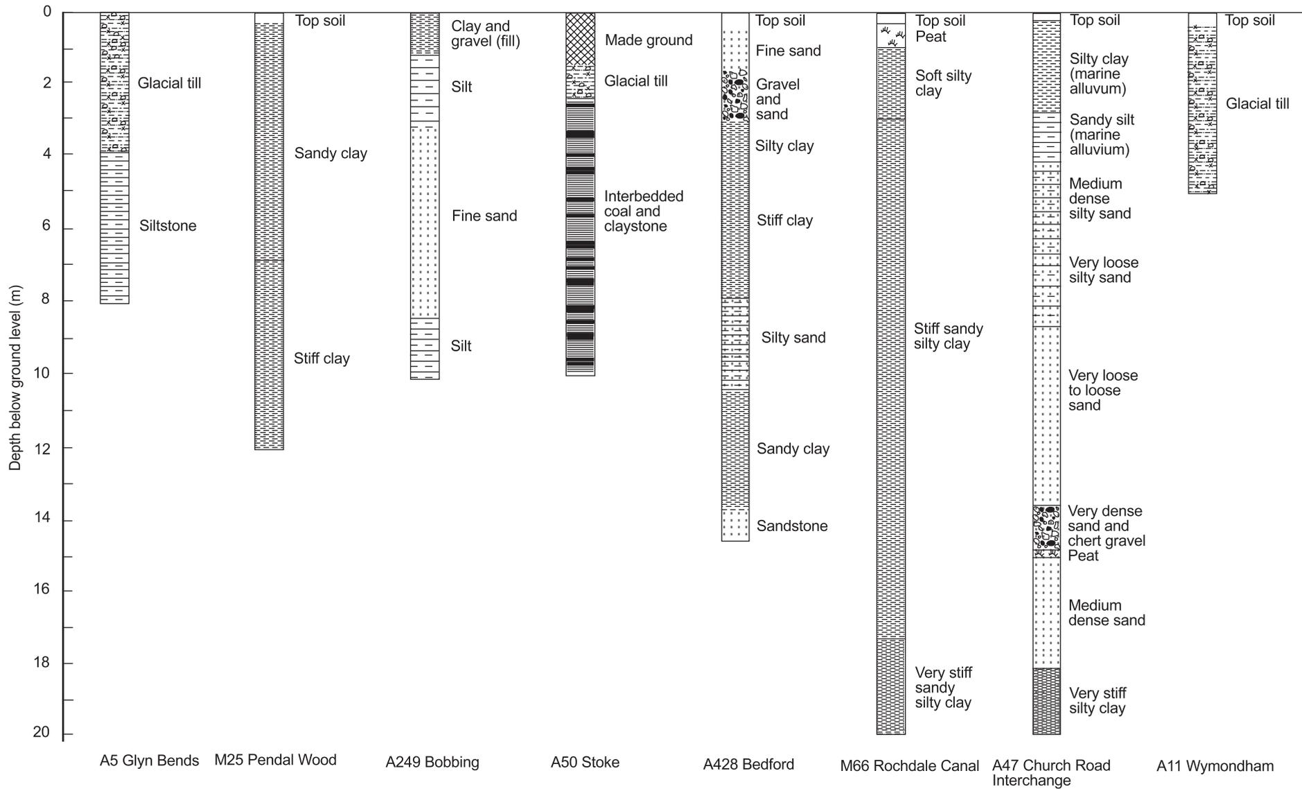
**Figure 9b** Simplified geological profiles for the remaining eight sites on which data from vibrating rollers were acquired
