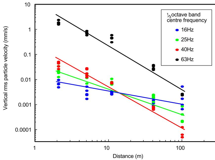
**Figure 24** Variation of rate of attenuation with vibration frequency
