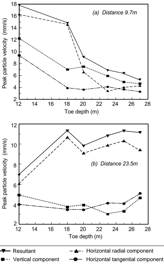
**Figure 35** Vibration data from Figure 34 for horizontal distances of (a) 9.7m, and (b) 23.5m from the pile
