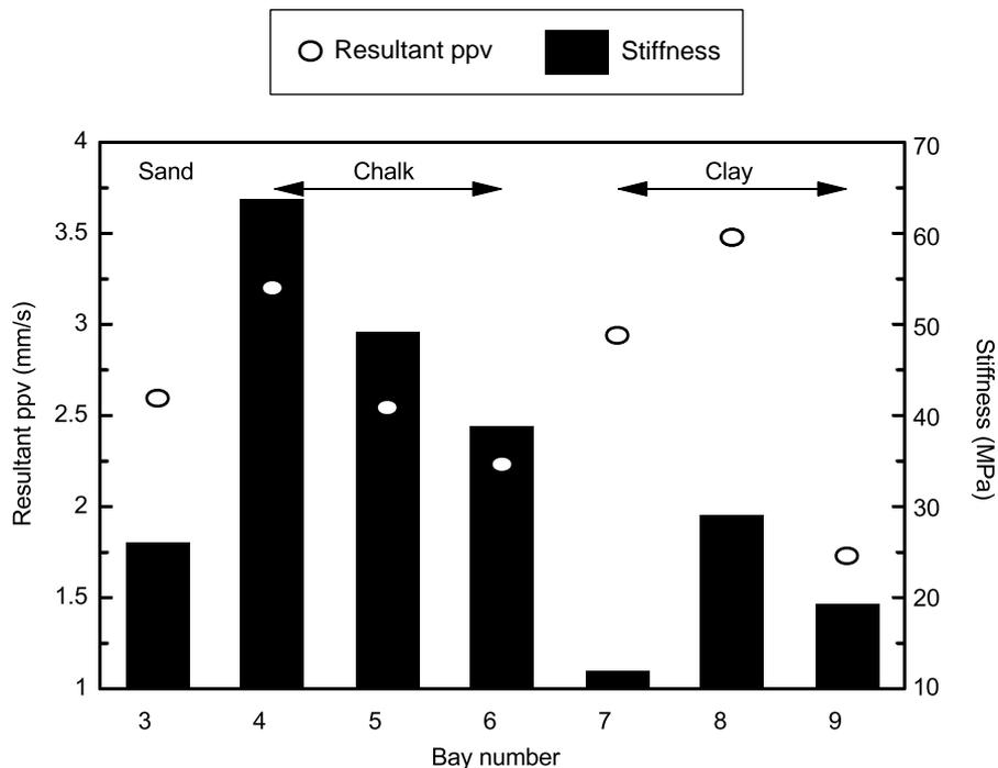
Section 22 Relation between the trial road subgrade stiffness and the ppv recorded at a distance of approximately 4m
