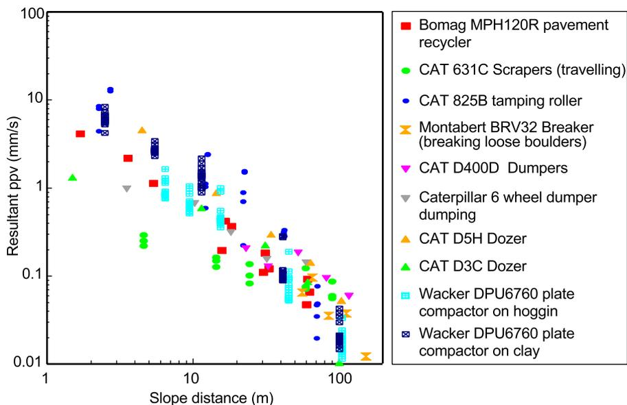
**Figure 50** Data acquired from miscellaneous operations on highway construction sites
